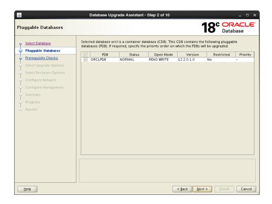
Starting in release 12.2, you can select the upgrade priority for PDBs. Click in the priority column for each PDB, and enter a numeric value for upgrade priority, where 1 is upgraded first, 2 is upgraded second, and so on.
